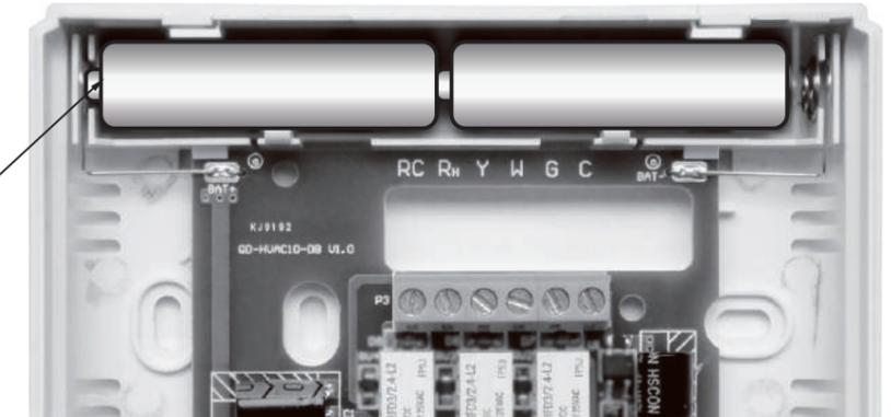
Insert 2 AA Alkaline batteries( not included ). High quality alkaline batteries are recommended.
