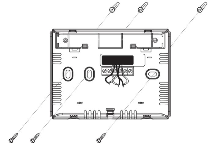
For horizontal mount put one screw left and one screw right.
