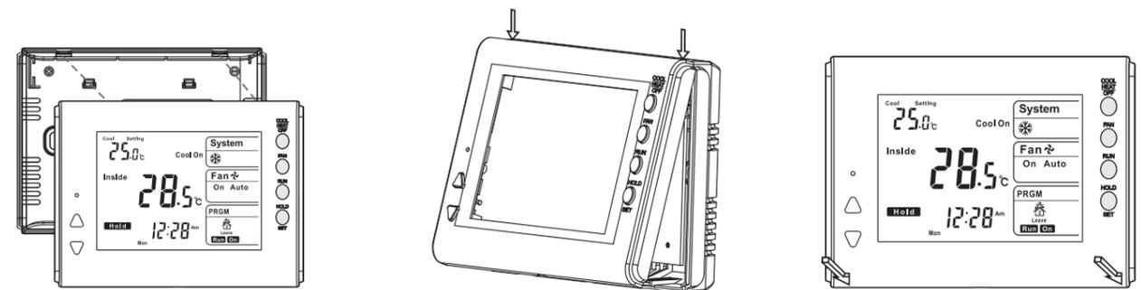
Step 1: Aim at the inner snaps in the higher part of the thermostat.
